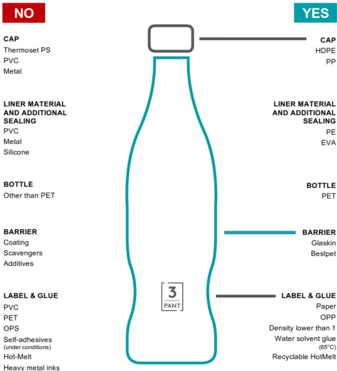
Figure 8 - Technical specifications for PET bottles (none of the NO materials is approved on any part of the bottle)<sup>18</sup>
